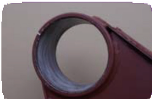
Fig. 9 - Lubricating the silentblock housing
