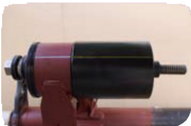
Fig. 14 - Correct position of the liner with the suspension arm
