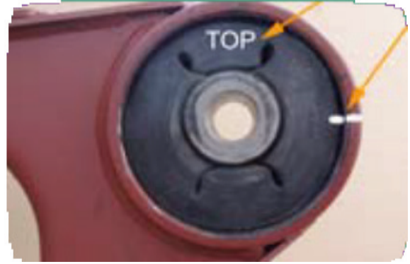
Fig. 17 - Checking for correct assembly
