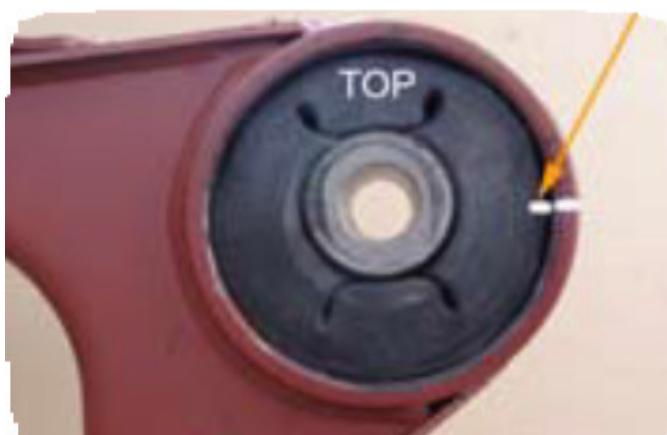
Fig. 4 - Close-up of the silentblock retraction position
